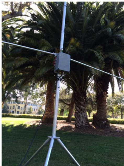
Tom Schiller Bravo 7K vertical antenna
