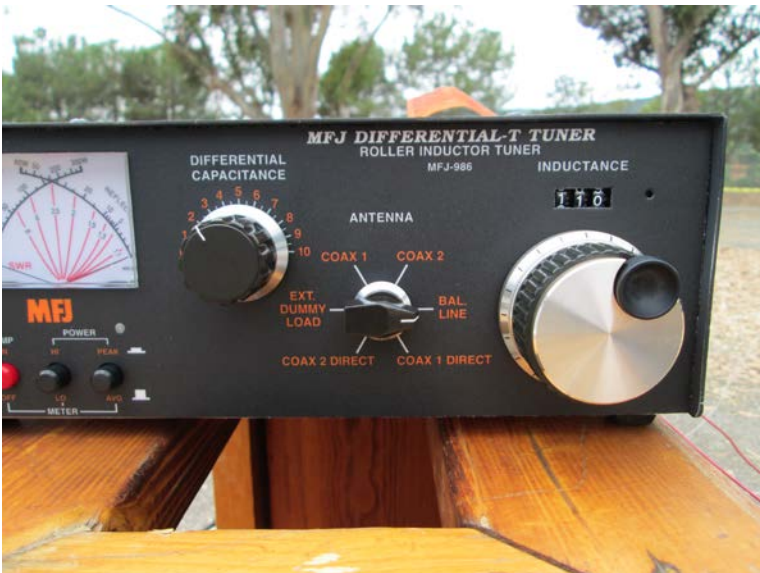
The MFJ 986 tuner was vital for tuning the balloon-lifted vertical long wire TX antenna for 160m and 80m.
