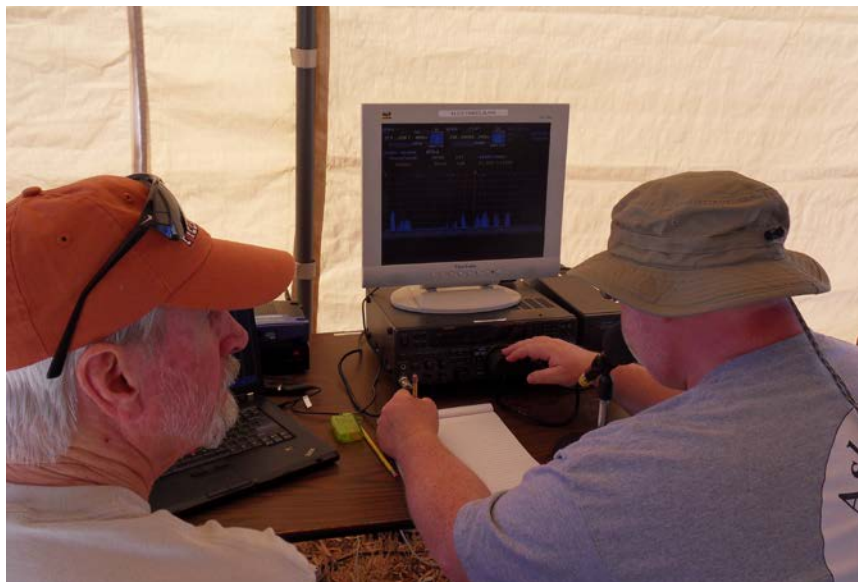
Above Photo: Dave W6VYC (left) and Michael NE6RD (right) team up to operate the SSB station. The station consists of a Yaesu FT-950 with a Yaesu DMU-2000 (pic at right). The Data Management Unit (DMU) connects to a monitor to provide a wide array of informative and useful displays, including a spectrum scope, grayline page and more. Above photo taken by Jeanette Dilley
