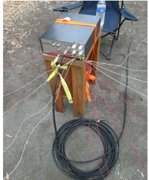
Tuner and radials for 160/80 meters
