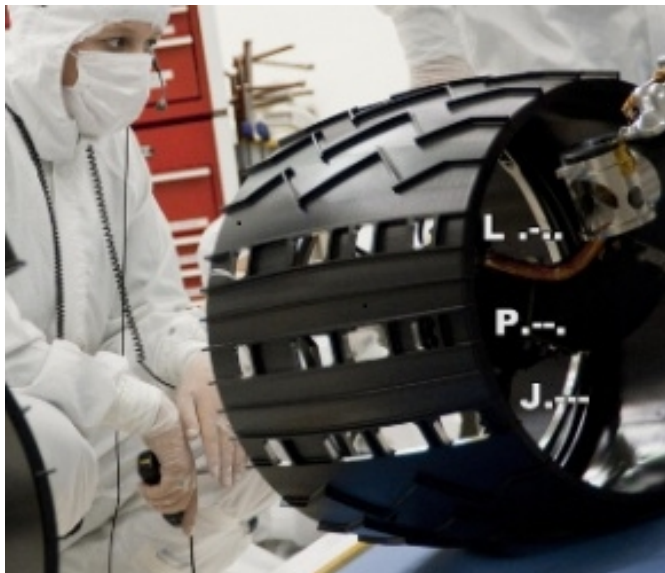
Detail of Mars Science Laboratory Curiosity Rover with tread pattern that will leave an impression on the Martian surface spelling "JPL" in Morse Code (· --- · --- · ---). Photo courtesy of NASA/JPL.
