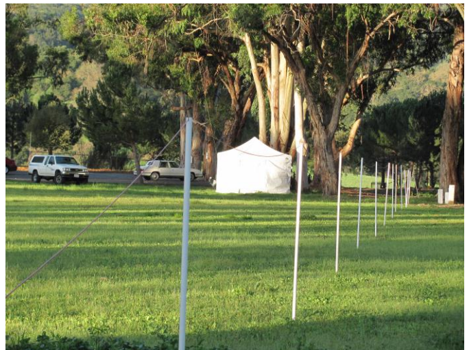
Beverage Antenna for receive on 160-Meters
