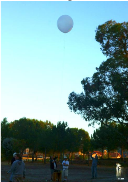
A large helium balloon is launched into the air to support a vertical tx antenna for 160m.
