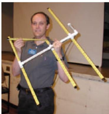
First Place (\$40) went to Mark Hardy, KG6GRR (that's me!). Mark made a 3 element YAGI antenna using PVC pipe and elements cut from a tape measure – titled the "Tape Measure Beam." It is light and rugged. Testing after the meeting showed the beam to be quite directional.
