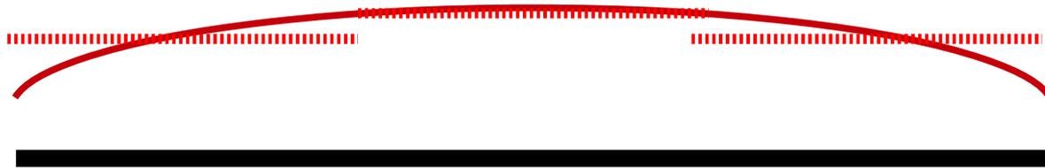
Model the real conductor with several “unit” antennas.
