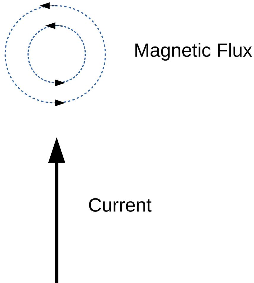
**Magnetic field forms concentric circles around the wire.**
