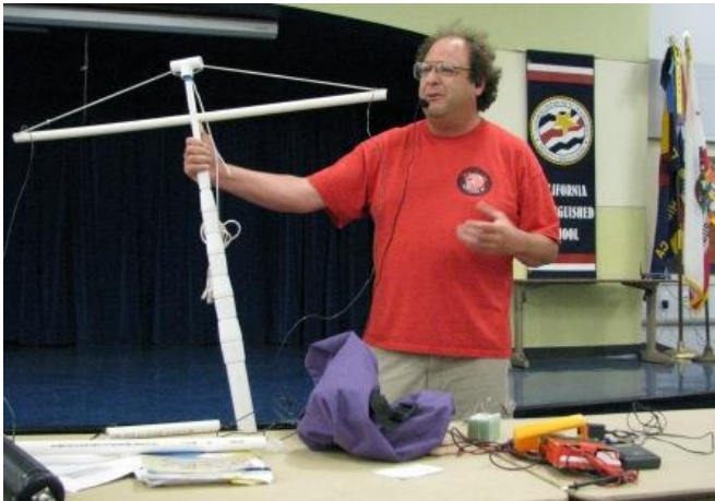
Cliff Sojourner, K6CLS, 20 Meter C-Pole (Do a web search for 20 meter C pole for instructions, also in the Antenna Designers Handbook)
