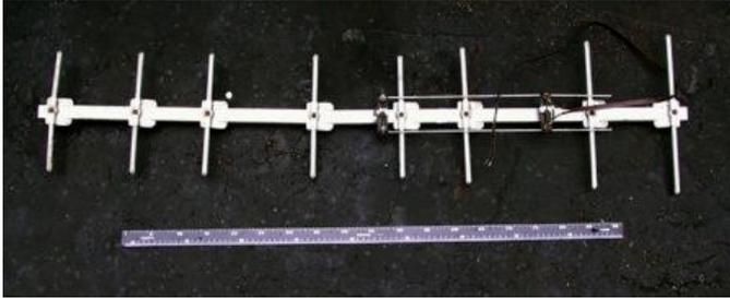
The picture shows 8 elements on a boom about 40 inches long. The other picture shows what should be the feed assembly. Just ahead of element 5 is a plastic insulator holding two screws with wing-nuts. Connected these screws and parallel to the boom are two metal rods. The rods extend past element 7. The dimensions and spacing compute to be a transmission line of 440 Ohms.
