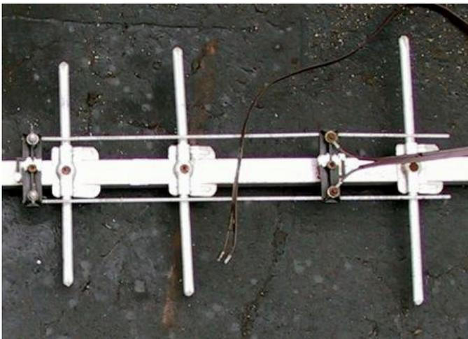
Between elements 6 and 7 is another plastic insulator. Under the nuts are terminal lugs holding a piece of 300 Ohm twin lead. Both ends of the twin lead have factory crimped connectors. At the second insulator, the nuts are regular hex nuts, not wing nuts. Where the wing nuts intended as the place to attach the feed line down the mast? Was the other piece of feedline intended to connect to another part of the antenna?
