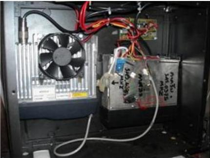
Here is the inside of the repeater controller station. They used a Motorola for receiving and an ICOM for transmitting. The controller has a simple circuit to take care of the audio and COS signal for PTT. The fan was running full time.
