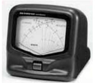
and output power simultaneously. Compact size makes it very useful for testing mobiles as well as base station installation. Features: Cross needle design, rated from 144-470 MHz, power ranges of 30 and 300 Watts.
