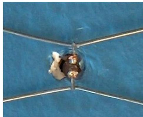
8. Pass the speaker wire transformer through the foam and solder to the center wire stubs. Make the final total length of the transformer to be 1 inch, the same as the foam thickness, with 3/4 inch of insulation still remaining in the middle of the transformer. If you are using a newer type of N connector with about 1/8 inch of connector sticking out beyond the flange (as shown in step 3 above), then the transformer will be bowed slightly in the hole in the foam.
