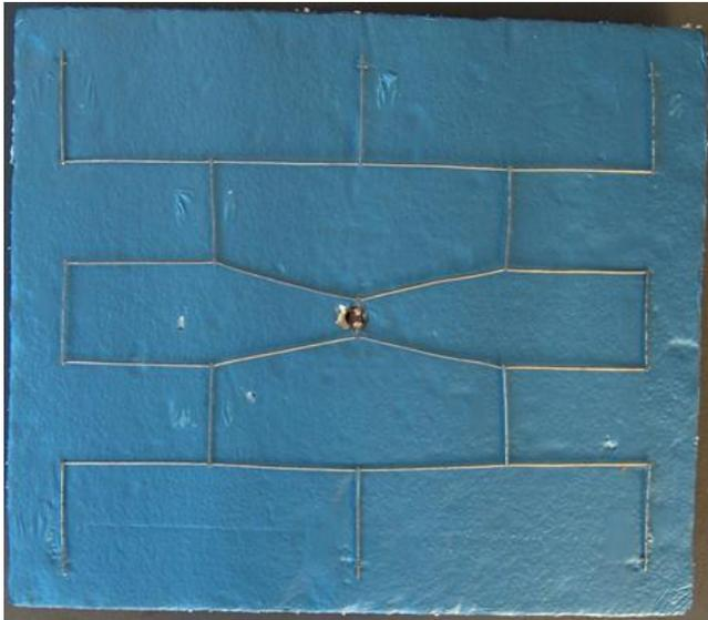
9. Secure the mounted connector to the back of the antenna with duct tape or aluminum backed tape.
