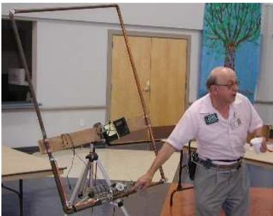
KR6DD, Andy, Full HF-band loop antenna
